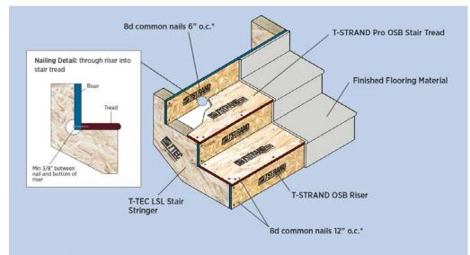
\*Predrill tread end grain at mid-thickness with 3/32" bit. Maintain at least 3/8" edge distance in riser.
