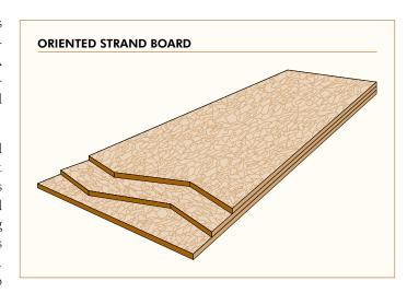
Most OSB sheathing panels have a nonskid surface on one side for safety on the construction site.
