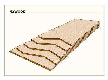
the grain oriented parallel to the long dimension of the panel.
