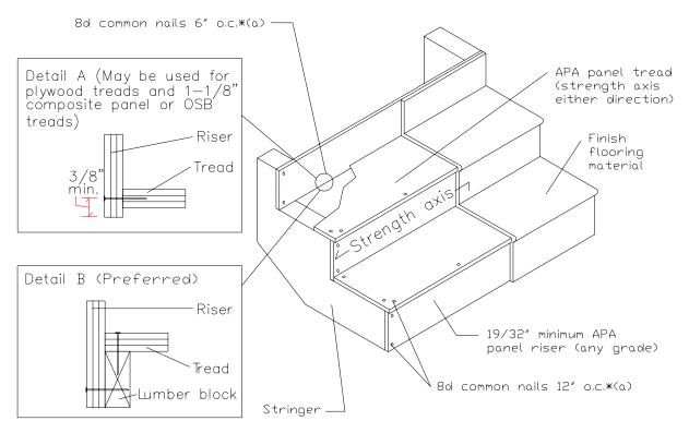
\*Predrill tread end grain at mid-thickness with 3/32'' bit. Maintain at least 3/8'' edge distance in riser.
