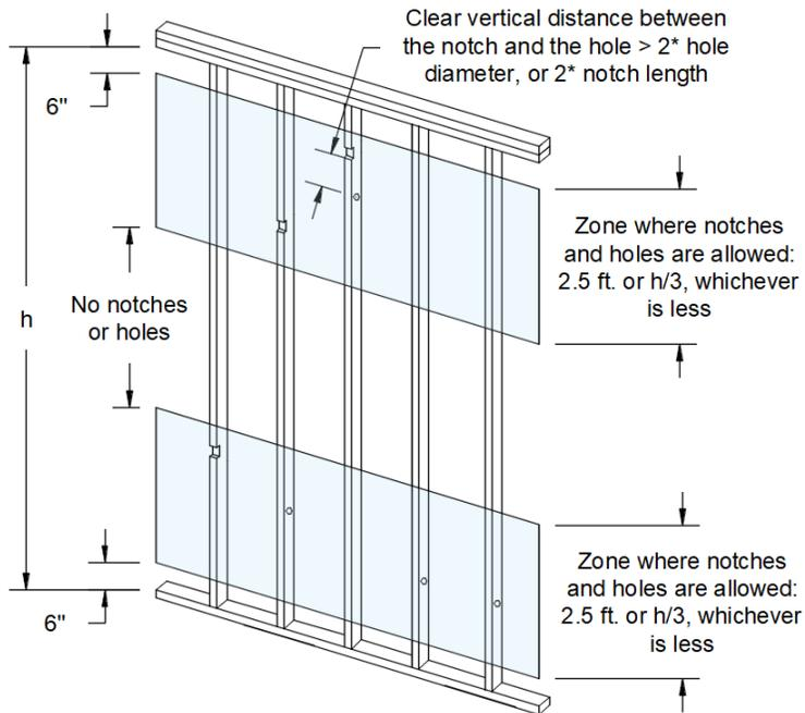
**Detail 16. Allowed Drilling and Notching Zones**
