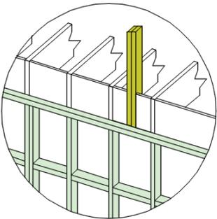
**TABLE 50: MAX. CONCENTRATED LOAD (lbs) TRANSFERRED BY THE 1.35E TOLKO T-TEC LSL TOP PLATE**
