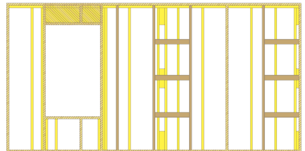
Advanced vs. Conventional Framing
